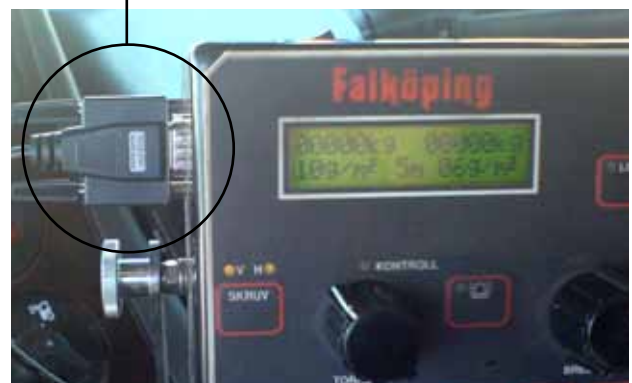
Connecting "Falköping" to the Magic box with a serial cable female to male
